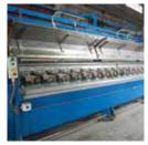
This European multi-wire drawing machine has a high production capacity by producing multiple wires at the same time. It is able to maintain high productivity while maximizing the electrical properties of the wire.
