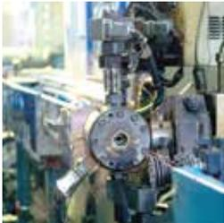
This European extrusion machine ensures that the insulation's electrical property and dimension are maximized. Problems such as off-centering, inconsistency of thickness, over or under burning of insulation materials are prevented with this machine.
